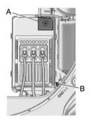
Your vehicle is equipped with a remote positive (+) terminal (A) and a remote negative (-) terminal (B). The remote
